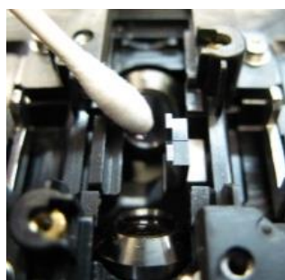
Detachable V-groove and Easy Cleaning
